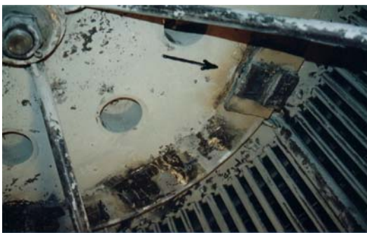
Figure 27: Balance Weights Inside Cage (Looking Toward Top of Cage)
