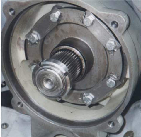
Figure 12: Spline on Power Turbine
