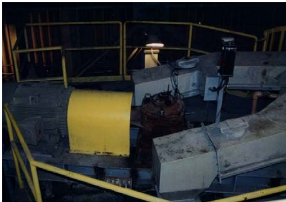
Figure 22: Motor and Right-Angle Gearbox
