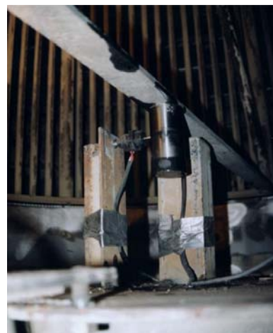
Figure 26: Potentiometers Used for Balancing Cage
