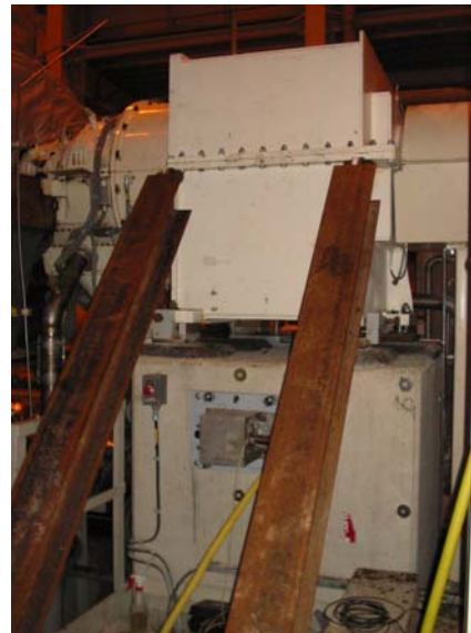
Figure 35: Clutch Box Diagonal Bracing
