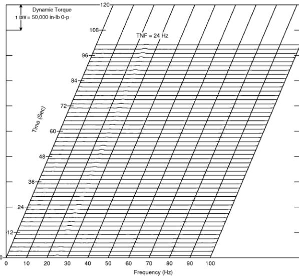
Figure 21. Time Waterfall Plot of Dynamic Torque with Motor Across the Line.
