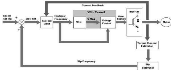
Figure 3. Block Diagram for Volts/Hertz. (Courtesy of Rockwell Automation, 2000)
