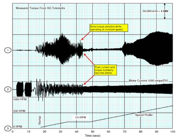
Figure 24. Time Traces from Test Run 1.
