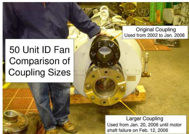
Figure 5. Comparison of Coupling Sizes.
