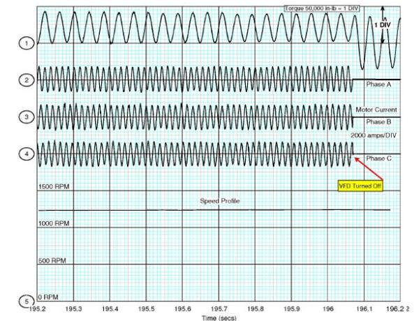
Figure 20. Time Wave Forms as VFD was Switched Off.
