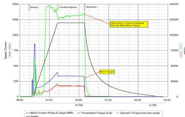
Figure 13. Trend Plot at Maximum Speed of 1197 RPM.
