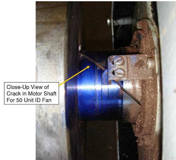
Figure 16. Crack in Motor Shaft.
