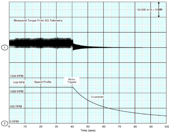
Figure 26. Trip Event and Coastdown at End of Test Run 1.
