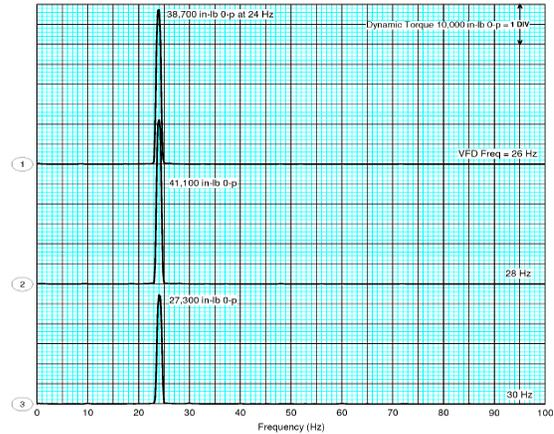
Figure 33. Frequency Spectra of Dynamic Torque with New VFD.
