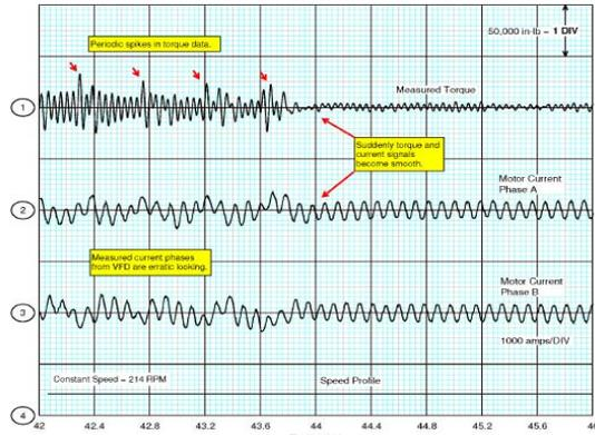
Figure 25. Measured Torque and Motor Current Versus Time.
