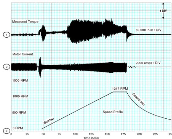
Figure 18. Time Traces and Speed Profile Taken During Startup.
