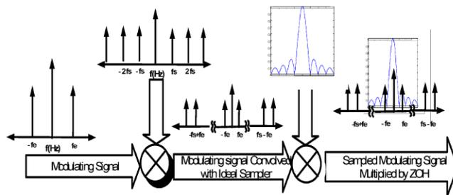
Figure 29. PWM Model Showing Spectrum Smearing. (Courtesy of Kerkman, et al., 2008)
