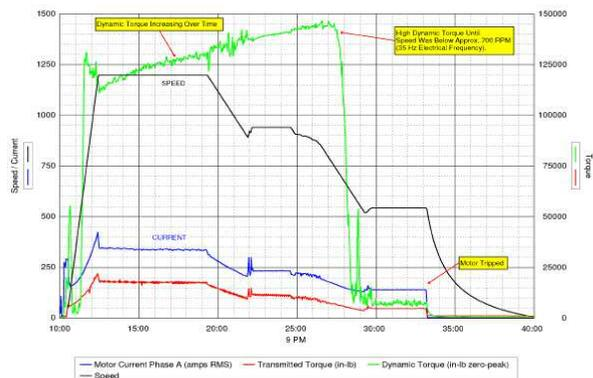
Figure 10. Trend Plot with Inlet Dampers Closed.
