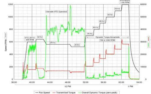
Figure 32. Trend Plot from Multiple Speed Test with New VFD.
