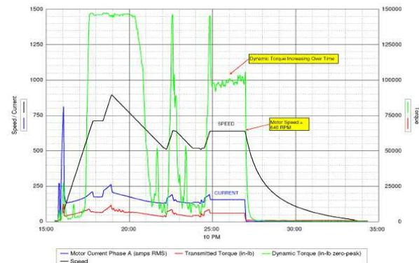
Figure 12. Trend Plot as Fan Speed Varied with Dampers Closed.
