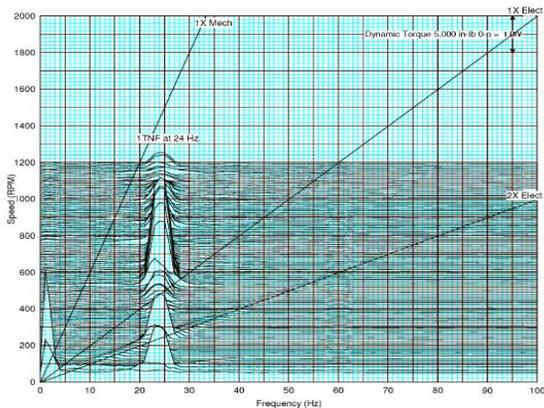
Figure 30. Waterfall Plot of Dynamic Torque with New VFD.
