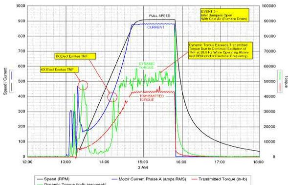
Figure 8. Trend Plot with Inlet Dampers Open.
