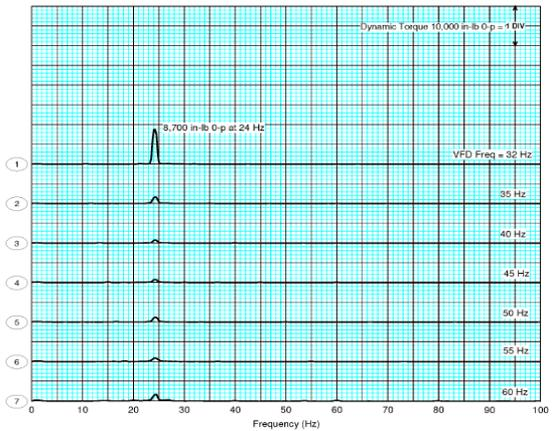
Figure 34. Frequency Spectra of Dynamic Torque with New VFD (Continued).
