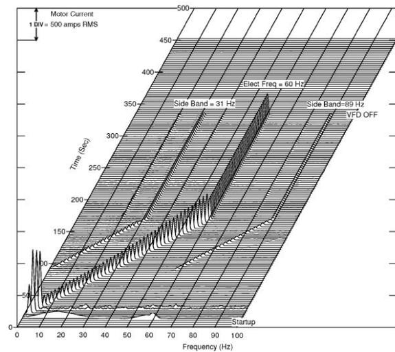
Figure 14. Time Waterfall Plot of Motor Amps.
