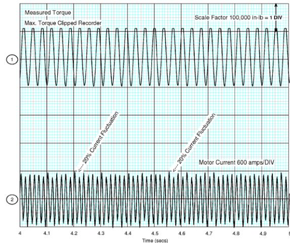
Figure 11. Time Traces with the Fan Operating at 1197 RPM.
