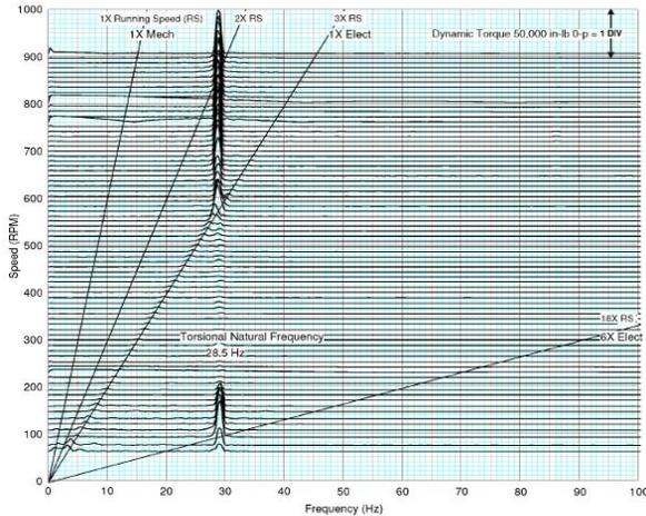
Figure 7. Waterfall Plot of Dynamic Torque During Startup.
