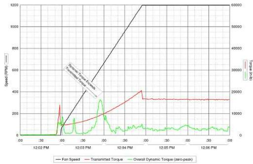
Figure 31. Trend Plot Taken During Startup and Operation with New VFD.
