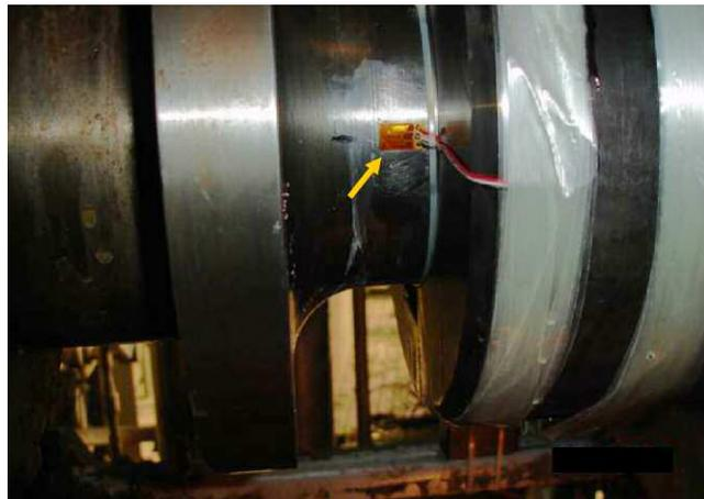
Figure 6. Strain Gauge Telemetry System.
