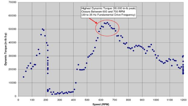
Figure 23. Plot of Dynamic Torque Versus Speed.
