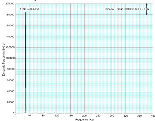
Figure 15. Frequency Spectrum of Dynamic Torque During Normal Operation with Furnace in Service.
