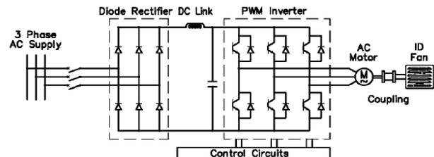
Figure 2. Components of VFD. (Courtesy of Barnes, 2003)
