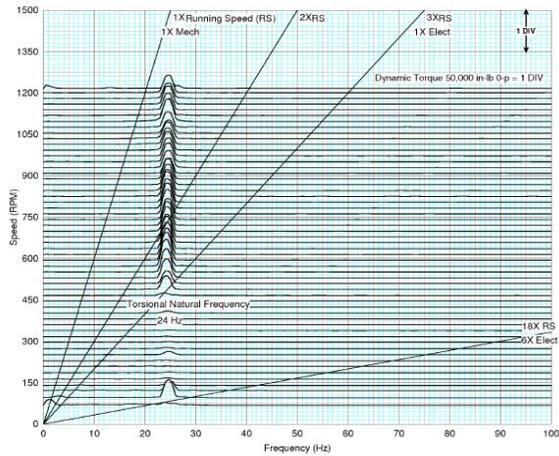
Figure 17. Waterfall Plot of Dynamic Torque During Startup.
