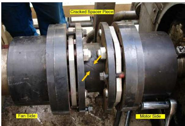
Figure 4. Cracked Coupling Spacer.
