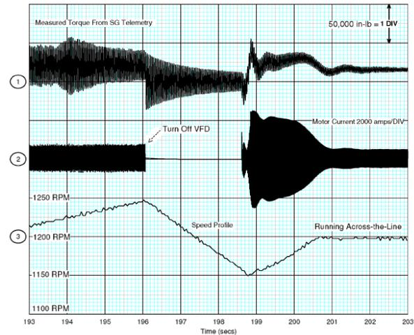
Figure 19. Switch to Across-the-Line Operation.
