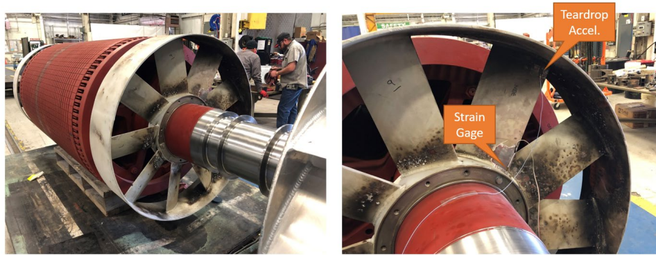
Figure 19. Close-Up of Internal Fan NDE with Instrumentation
