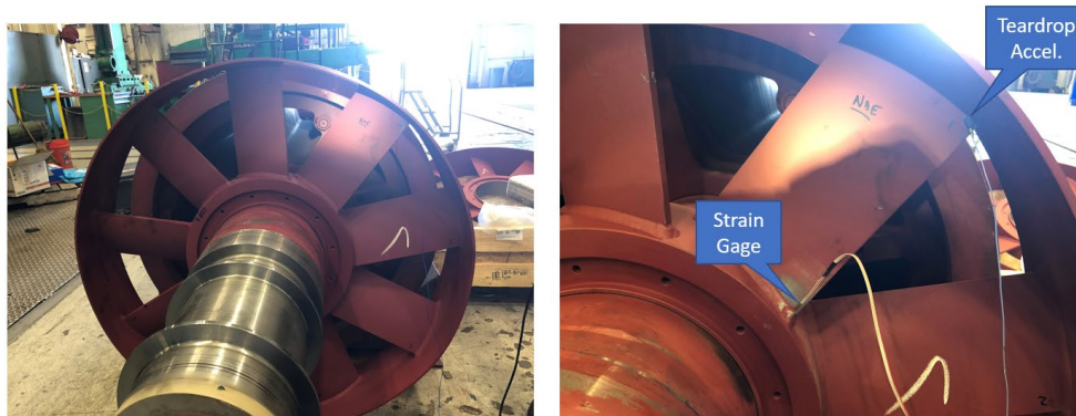
Figure 22. Close-Up of Internal Fan NDE with Instrumentation
