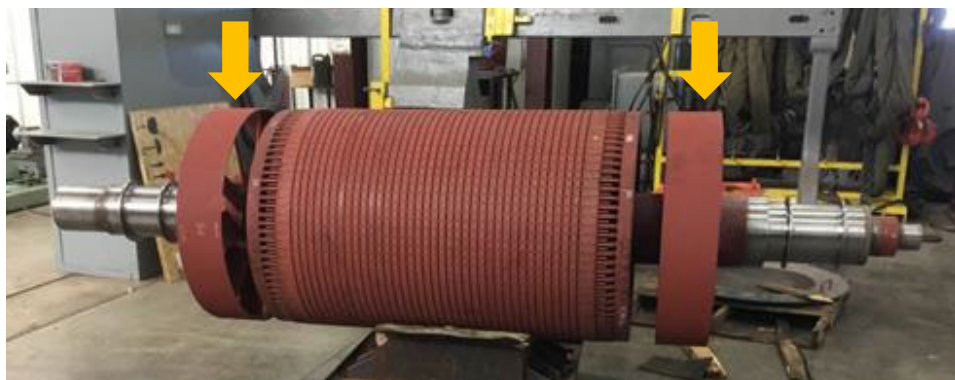
Figure 17. Motor Rotor with Internal Fans
