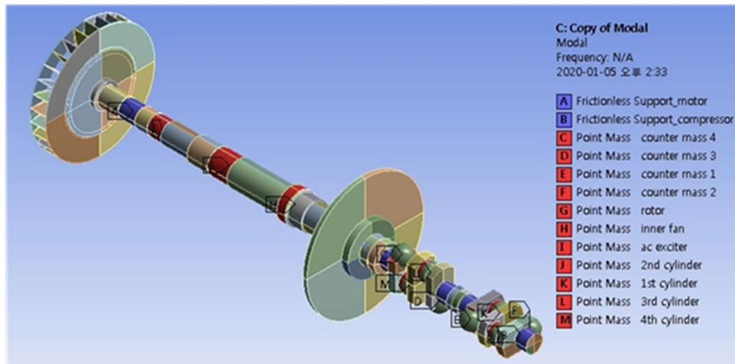
(c) Torsional system consisting of crank and motor shaft with additional inertia elements including external cooling fan
