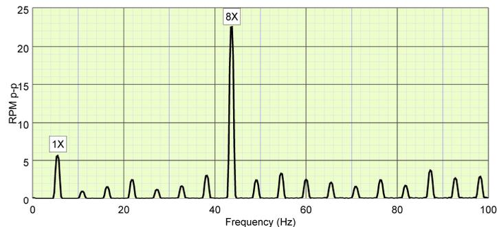
(b) Speed fluctuation of motor fan
