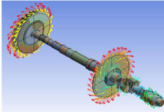
(a) 1<sup>st</sup> torsional mode at 45.0 Hz (40.0 Hz after modifications)
