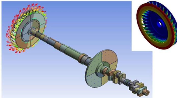
(b) 2<sup>nd</sup> torsional mode at 58.4 Hz (56.1 Hz after modifications)
