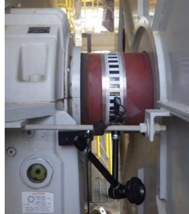
Figure 4 – Laser and zebra tape installed on the motor shaft between bearing and external cooling fan
