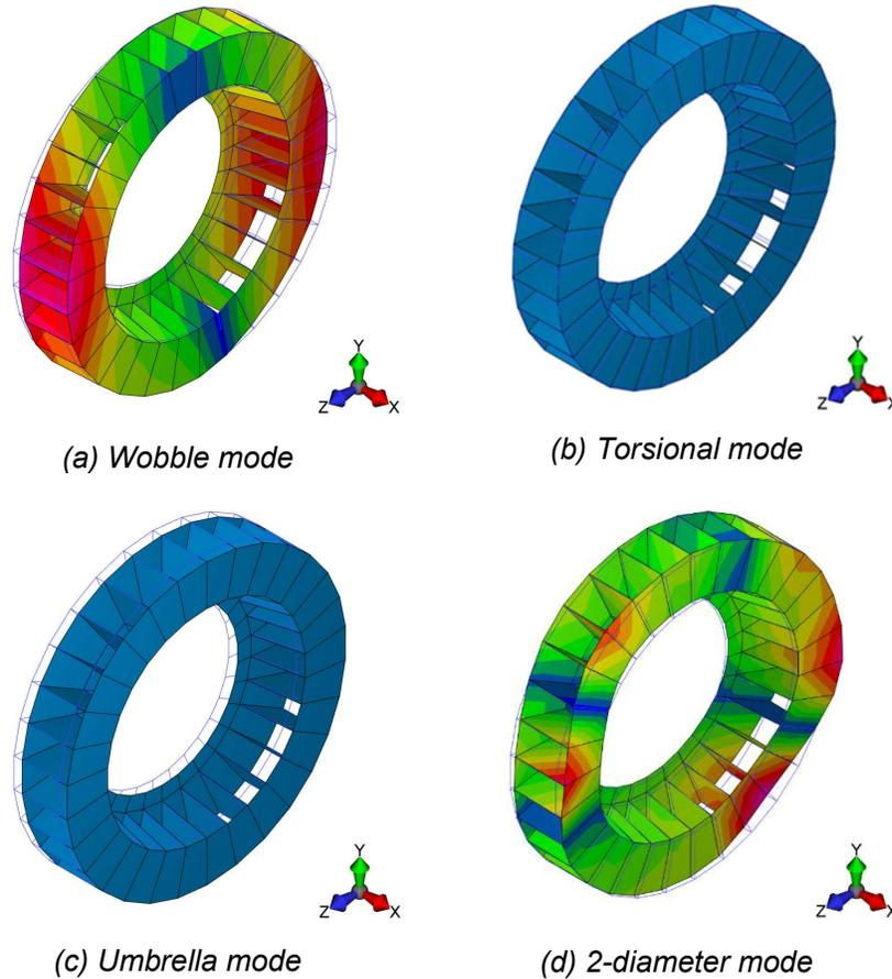
Figure 3 – IMS results of external cooling fan
