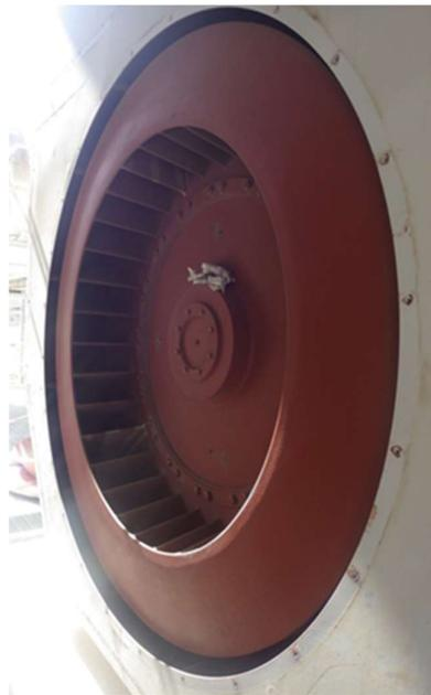
*Figure 2 – External motor cooling fan*
