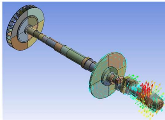
(c) 3<sup>rd</sup> torsional mode at 72.3 Hz (69.8 Hz after modifications)
