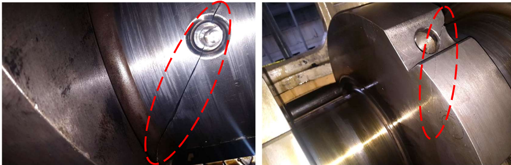
Figure 3. Photos of cracks in engine crankshafts
