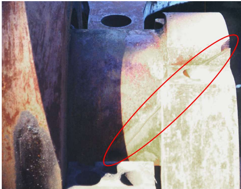
Figure 1. Failed Engine Crankshaft without Damper
