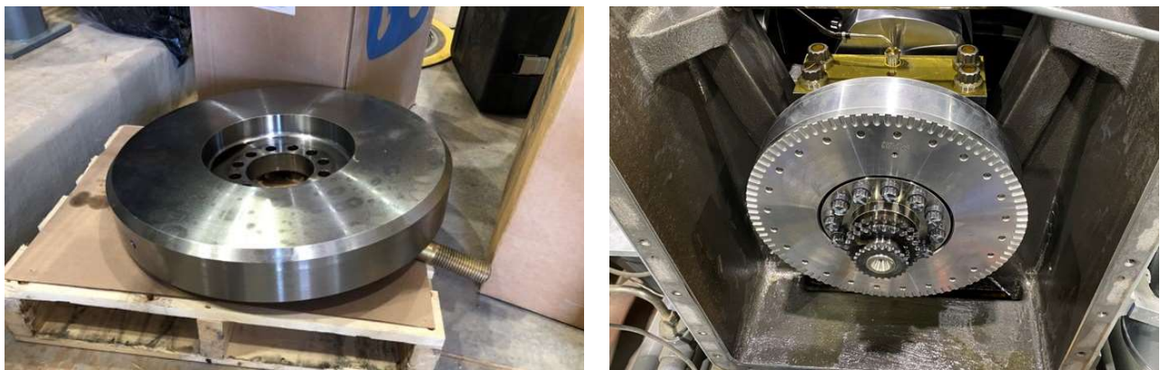
Figure 18. Internal Flywheel (left) and Internal Damper (right)
